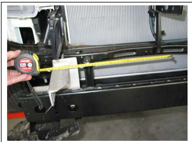
Figure 5 – Drivers side shown centralising steel mounting bracket
