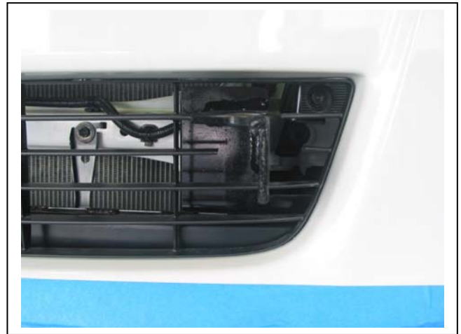
Figure 12: Trim grille to suit placement of mounts
